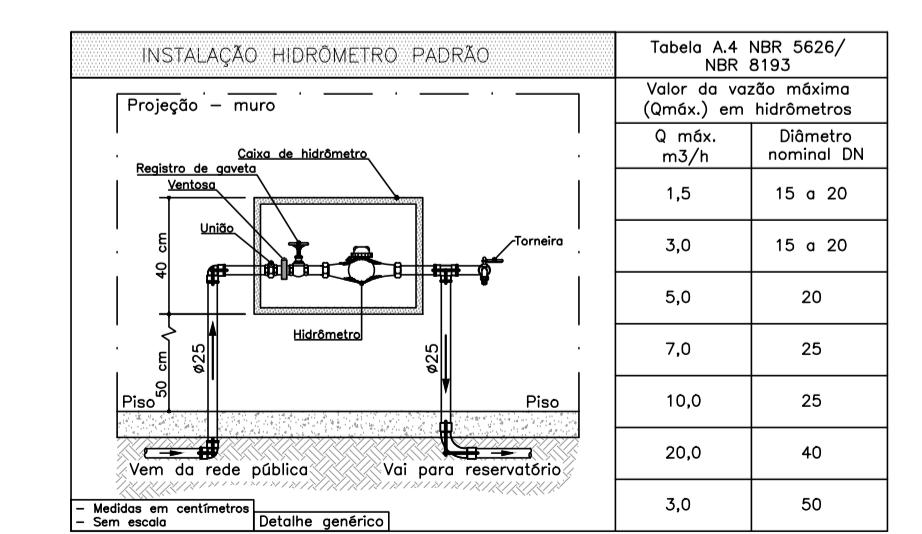
DETALHE 01 - CAVALETE HIDRÁULICO
